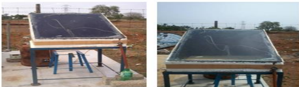
Figure.3. Photographic view of conventional solar still and basin with titanium dioxide
