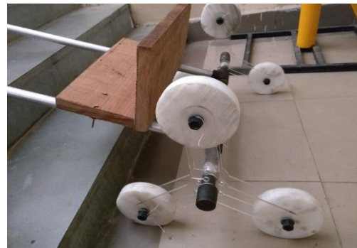
Figure. 6(b). Close-up of the Tri-Star wheel in the Working Prototype
