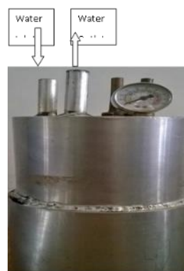
Figure 1. Assembly of Cavity Receiver Figure 2. Receiver machined from Aluminium Bar
