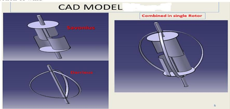
Fig 1 CAD Model of Savonius, Darrieus, Combined Turbine.
