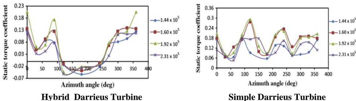
Fig 2 Static torque Co efficient vs. azimuth angle of Simple H Rotor at Reynolds no.  $1.44 \times 10^5$ (7.5m/s),  $1.60 \times 10^5$ (8.33m/s),  $1.92 \times 10^5$ (10m/s),  $2.31 \times 10^5$ (12m/s)
