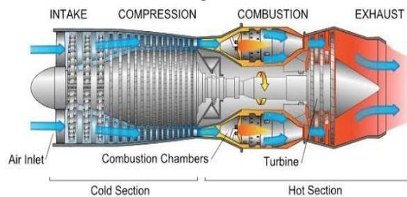
**Fig.3. Gas turbine operation**
