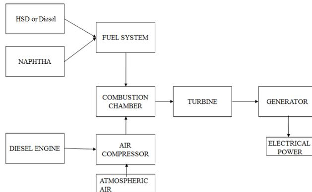
**Fig.5. Basic block representation for the operation of gas turbine**
