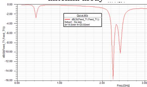
Figure.7. Return loss of the series-feed microstrip patch antenna array
