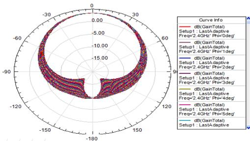
Figure.8. Radiation pattern of the single patch antenna
