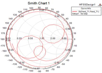
**Figure.10. Smith chart of the single patch antenna**
