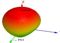
Figure.4. Gain of the single patch antenna
