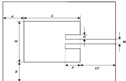
**Figure.1. Rectangular microstrip patch antenna**
