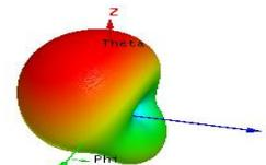
Figure.5. Gain of the series-feed microstrip patch antenna array
