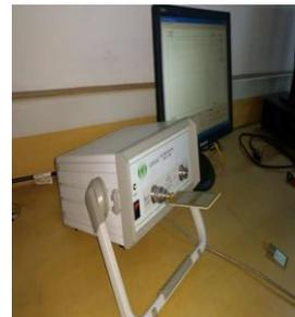
**Fig. 13. Testing of the microstrip Patch Antenna array in series-feed configuration using Network Analyzer**
