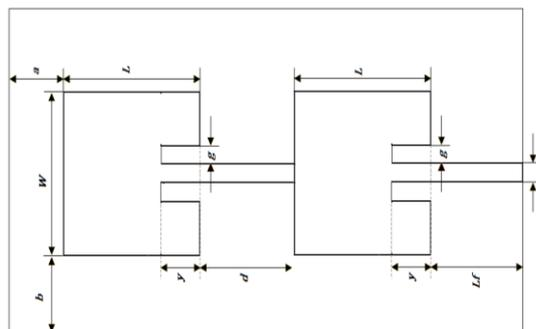
**Fig. 2. Series-feed microstrip patch antenna array or microstrip patch antenna array in radiating slot**
