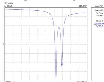
**Figure.15. Response of the microstrip patch Antenna array in series-feed configuration using Network Analyzer**
