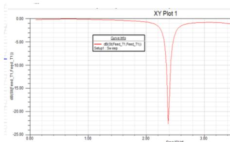
Figure.6. Return loss of the single patch antenna
