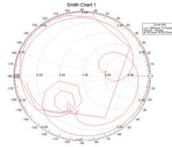
**Figure.11. Smith chart of the series-feed microstrip patch antenna array**
