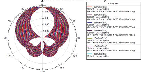
Figure.9. Radiation pattern of the series-feed microstrip patch antenna array
