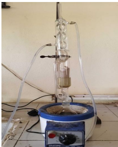
Figure 1: Soxhlet Extraction Apparatus Used for Extracting Nigella sativa Seeds.
