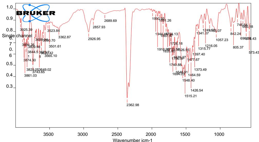
Figure 2: FTIR of pure drug Atorvastatin calcium
