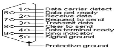
Figure.3. RS-232 connectors
