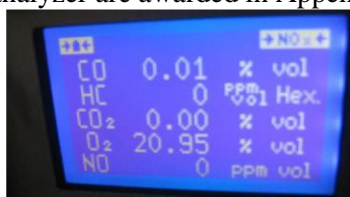
Figure.2. Measurement of exhaust gas analyzer
