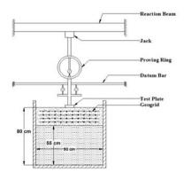
Figure.1. shows the test setup for granular soil as foundation bed
