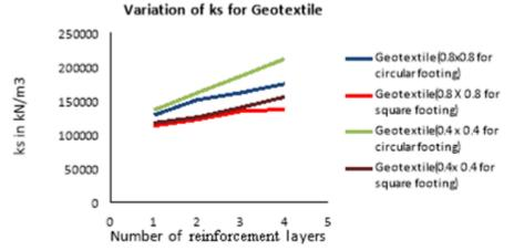
Figure.5. Values of  $k_s(kN/m^3)$  of weak soil using Plate Load test under model circular footing(100 mm ) and model square footing (100mm x 100mm)
